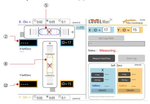
⑤ and ⑧ Display the bubble display when disconnected.
