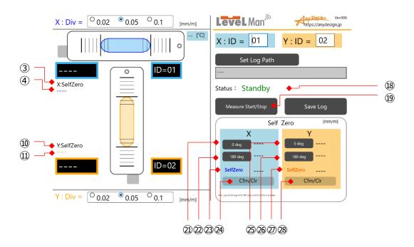
Self Zeroing calculates and saves adjustment deviations using the 180° inversion method. The correction value is then automatically applied to the measurement results.
