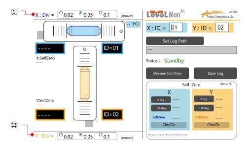
■ The scale sensitivity setting adjusts the bubble movement on the screen, allowing it to function like a level with different sensitivities.
