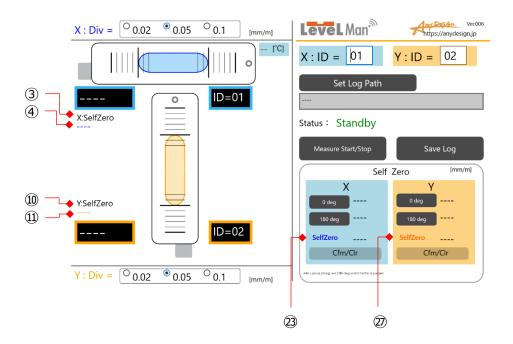
If the measured values in both the 0° and 180° positions are confirmed to be correct, press the ② [Cfm/Clr] button to save the correction value.
