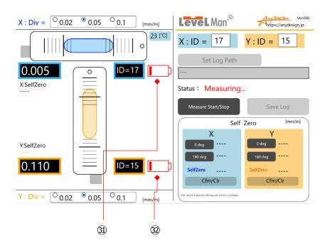
3 and 3 display low battery warnings for unit X and unit Y.
